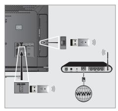
Connect Grundig WiFi USB dongle to the »USB« or »USB HDD« socket of your television in order to connect the television to a wireless network. Notes:
